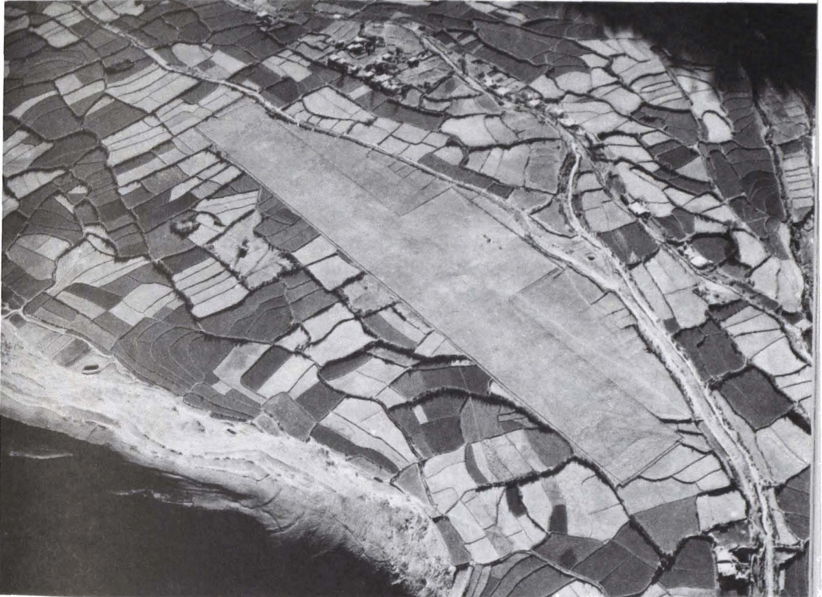
Fig. 42. Aerial view of the STOL airfield at Jumla-Kalanga. Occupying 4 ha of prime khet farmland on an alluvial terrace at 2,340 m, it is 500 m in length.
