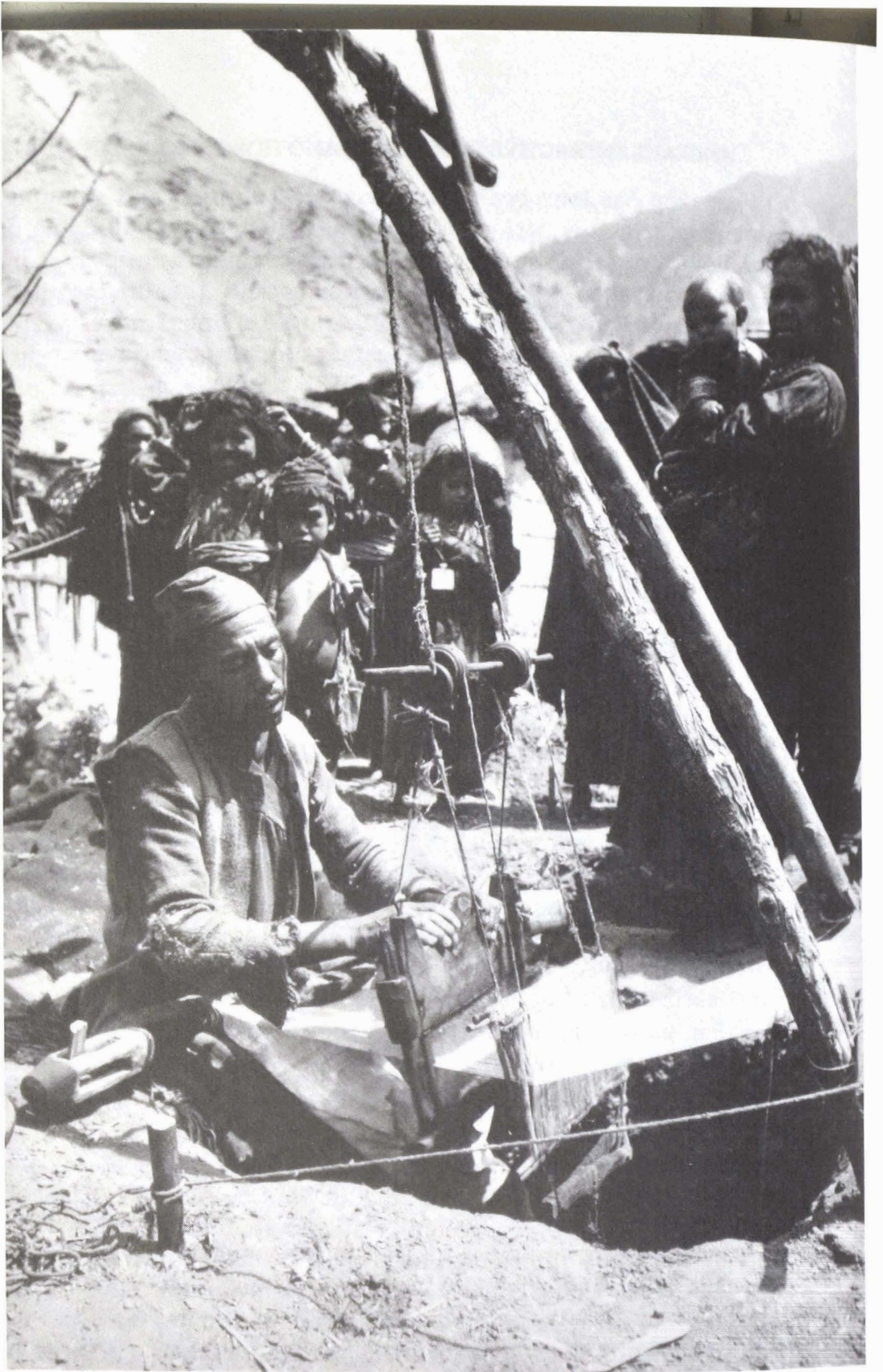
Fig. 70. Matwali Chhetri man weaving cotton cloth, or tetuwa. Such pit looms are commonly used in the Mugu Karnali Valley.
